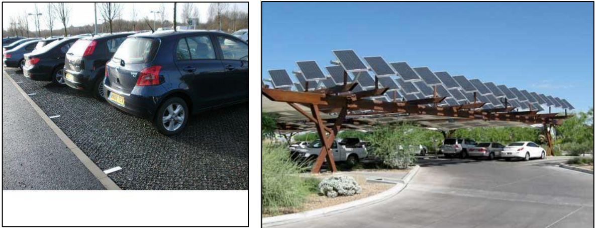
Fig 4: Examples of permeable paving (United Kingdom) and a solar parking lot (California)
